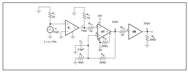
FIGURE 9. Simulation Circuit for Gauss Pulse Transmission (CG22DF2).
