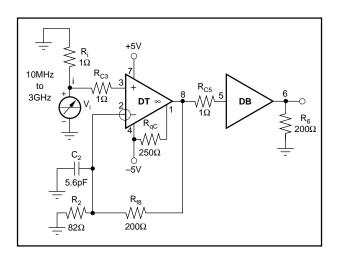
FIGURE 7. Frequency Response Analysis (CARDF2).
