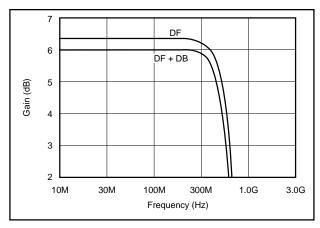
FIGURE 8. Simulation Result of the AC Sweep Response CARDF2.
