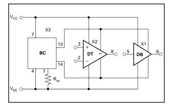
FIGURE 1. Block Diagram of the OPA660.
