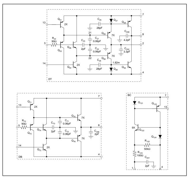
FIGURE 3. OPA660 Macromodel Consisting of the Subcircuits DT, DB, and BC.
