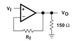
**-3dB Bandwidth vs Feedback Resistor Circuit Diagram**
