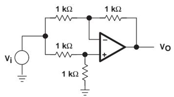
**Common-Mode Rejection Ratio Circuit Diagram**
