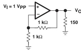
2nd and 3rd Harmonic vs Frequency Circuit Diagram
