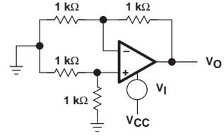
**Power Supply Rejection Ratio Circuit Diagram**
