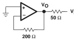
Z<sub>O</sub> Output Impedance Circuit Diagram
