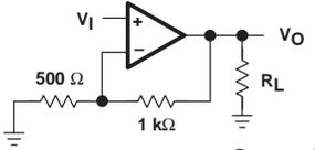
**Output Voltage (pp) Circuit Diagram**
