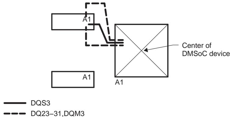
**Figure 11. General Data Byte 3 Routing**
