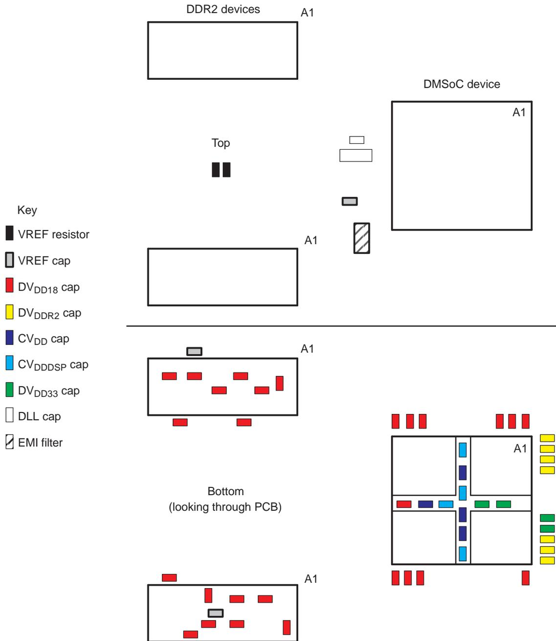
Figure 5. Discrete Part Placement
