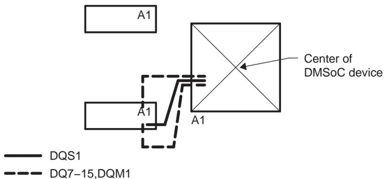
**Figure 9. General Data Byte 1 Routing**
