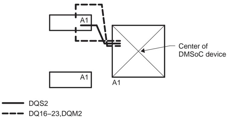
**Figure 10. General Data Byte 2 Routing**
