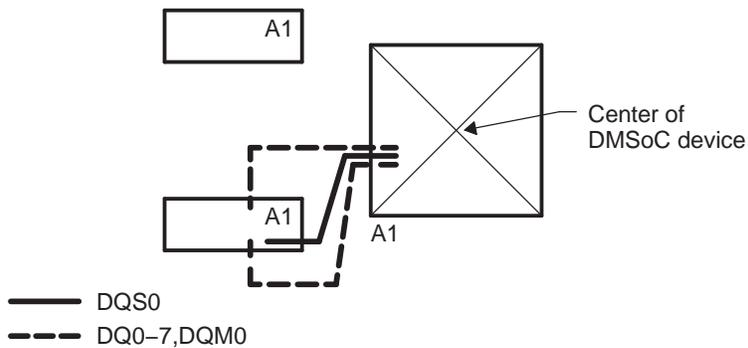
**Figure 8. General Data Byte 0 Routing**
