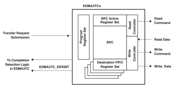
Figure 4. EDMA3 Transfer Controller Block Diagram
