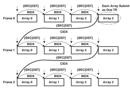
Figure 11. A-Synchronized Transfers (ACNT = n, BCNT = 4, CCNT = 3)
