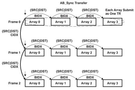
Figure 12. AB-Synchronized Transfers (ACNT = n, BCNT = 4, CCNT = 3)
