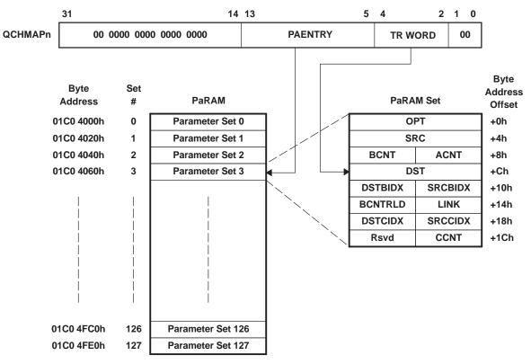
Figure 7. DMA and QDMA Channel Mapping to PaRAM
