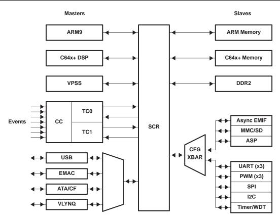
Figure 1. TMS320DM644x Device Block Diagram
