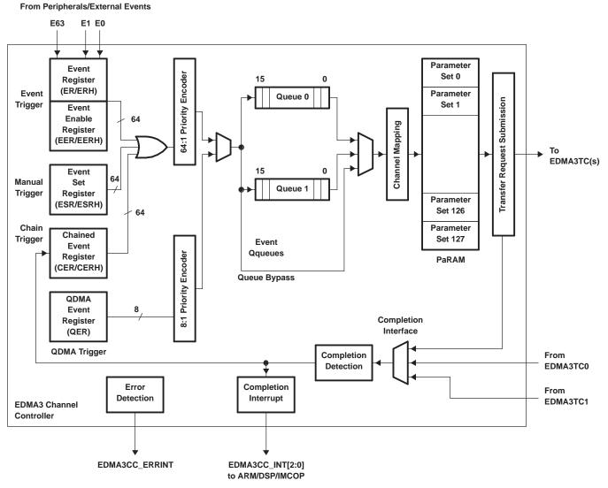
Figure 3. EDMA3 Channel Controller Block Diagram
