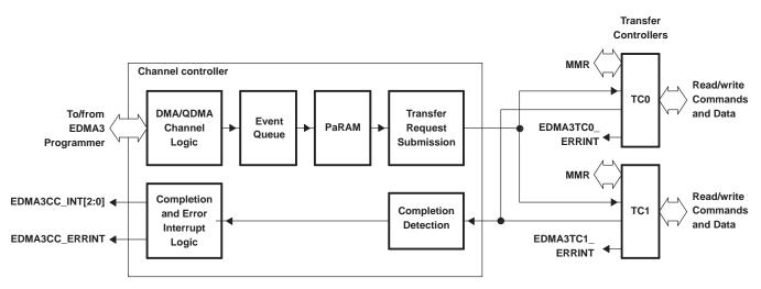
Figure 2. EDMA3 Block Diagram
