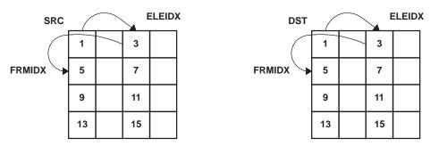
Figure 9. Indexing Example for EDMA2
