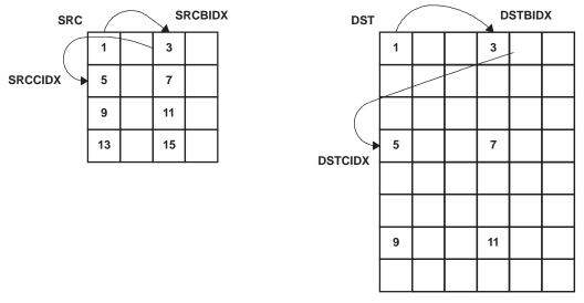
Figure 10. Indexing Example for EDMA3
