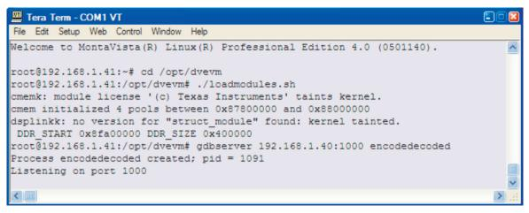
Figure 2. Tera Term Screen Showing Target DVEVM
