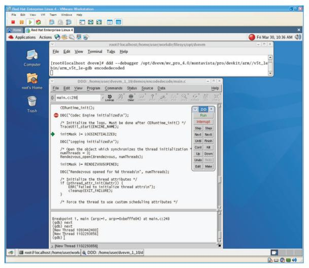
Figure 5. Breakpoints (stop sign) and Stepping Through Code (green arrow)
