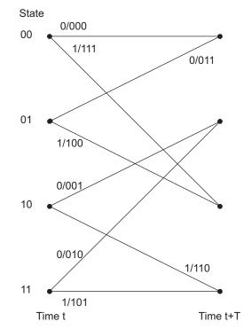
Figure 2. Trellis Diagram for Convolutional Encoder Example
