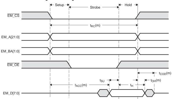
Figure 12. Timing Waveform of an ASRAM Read
