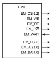
Figure 2. EMIF Asynchronous Interface
