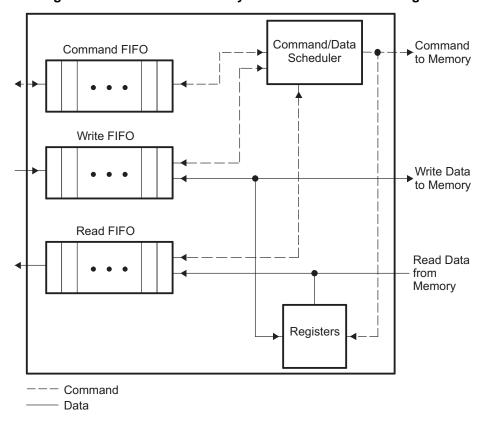
Figure 16. DDR2/mDDR Memory Controller FIFO Block Diagram
