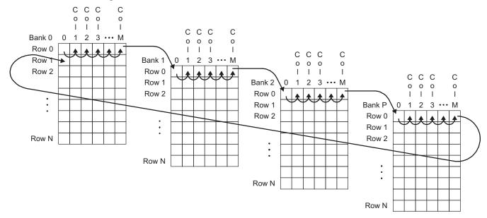
Figure 13. DDR2/mDDR SDRAM Column, Row, and Bank Access
