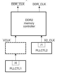
Figure 2. DDR2/mDDR Memory Controller Clock Block Diagram
