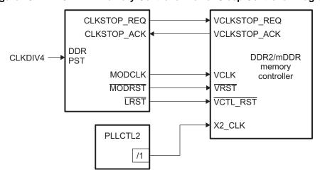
Figure 18. DDR2/mDDR Memory Controller Power Sleep Controller Diagram
