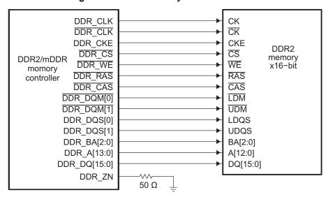
Figure 19. Connecting DDR2/mDDR Memory Controller to a 16-Bit DDR2 Memory
