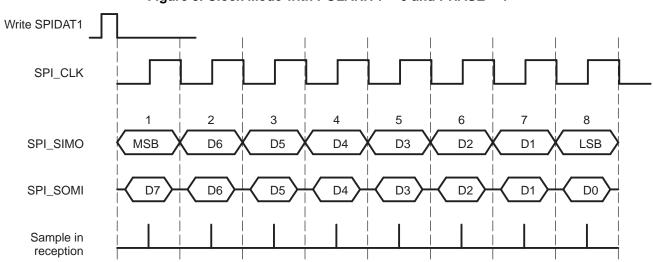
Figure 5. Clock Mode with POLARITY = 0 and PHASE = 1
