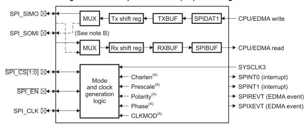
Figure 1. Serial Peripheral Interface (SPI) Block Diagram
