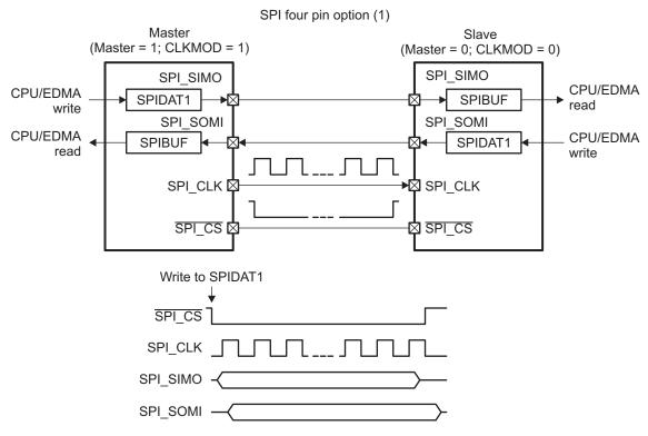
The SPI\_CS pins that are going to be used must be configured as functional in the SPI pin control register 0 (SPIPC0). The default pattern to be put on the SPI\_CS pins when all the slaves are deactivated is set in the SPI default chip select register (SPIDEF). This pattern allows different slaves with different chip-select polarity to be activated by the SPI.
