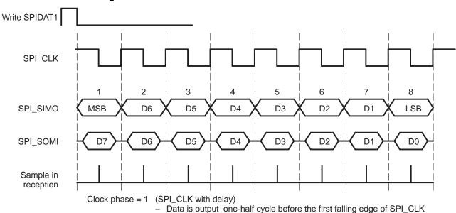
Figure 7. Clock Mode with POLARITY = 1 and PHASE = 1
