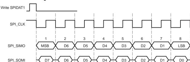
Figure 6. Clock Mode with POLARITY = 1 and PHASE = 0
