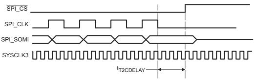
Figure 25. Transmit-Data-Finished-to-ENA-Inactive-Timeout
