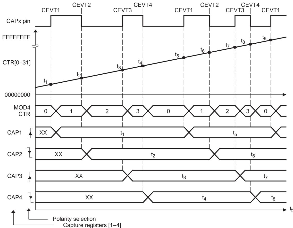
**Table 2. ECAP Initialization for CAP Mode Absolute Time, Rising and Falling Edge Trigger**
