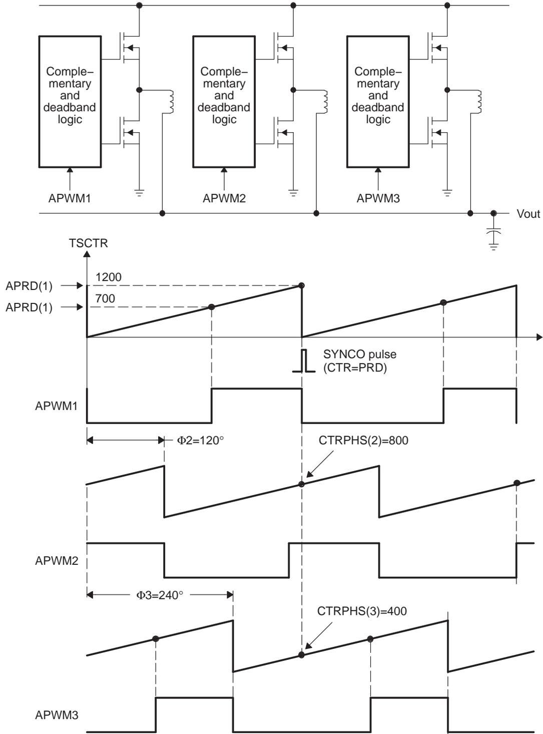
**Table 10. ECAP1 Initialization for Multichannel PWM Generation with Phase Control**
