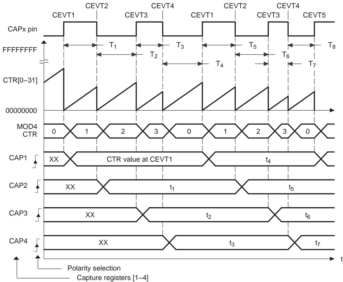
**Table 4. ECAP Initialization for CAP Mode Delta Time, Rising and Falling Edge Triggers**
