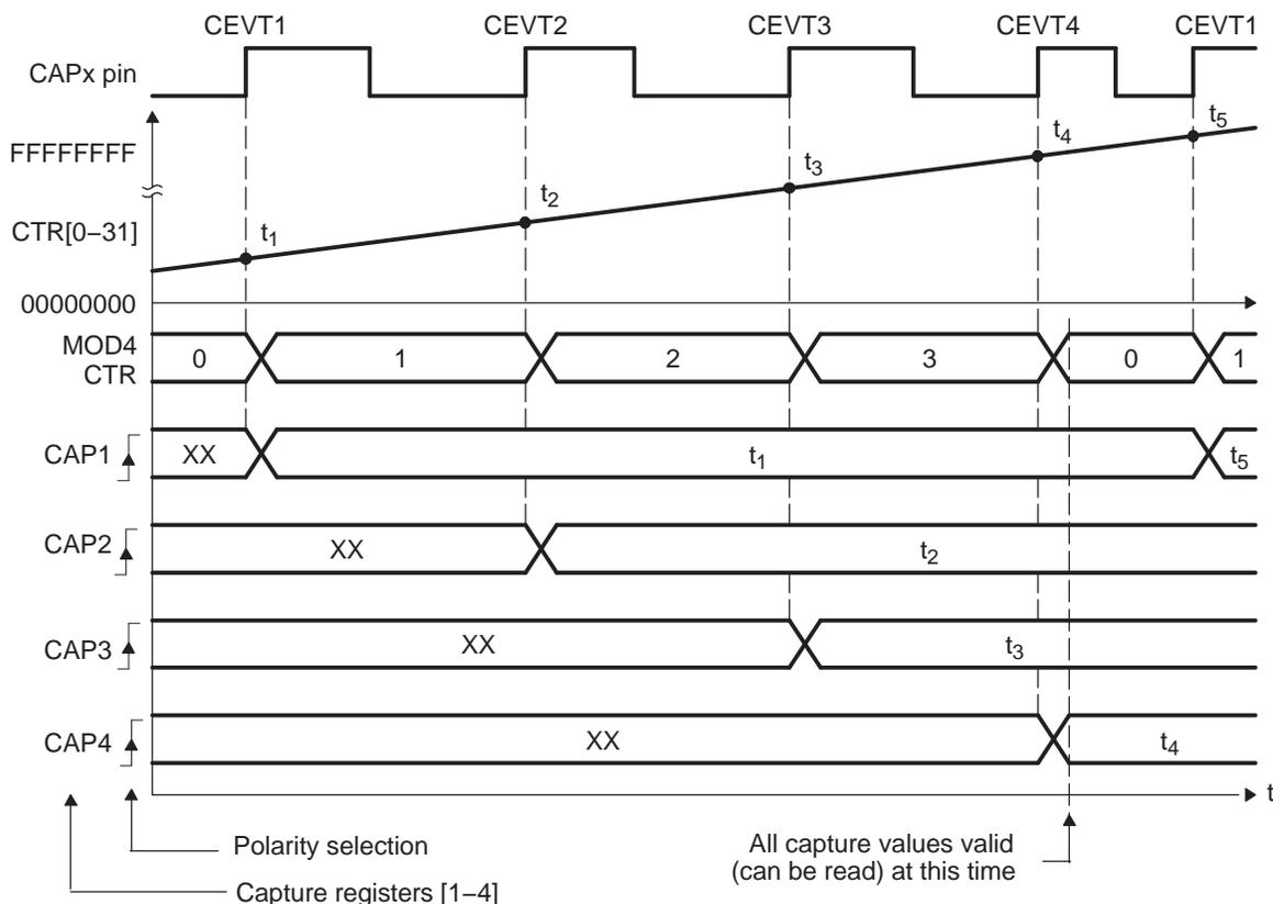
**Table 1. ECAP Initialization for CAP Mode Absolute Time, Rising Edge Trigger**
