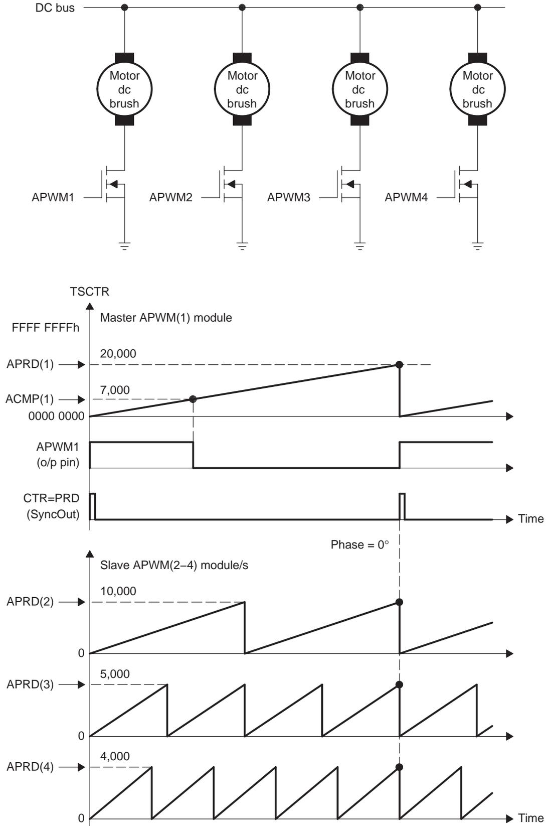
**Table 6. ECAP1 Initialization for Multichannel PWM Generation with Synchronization**
