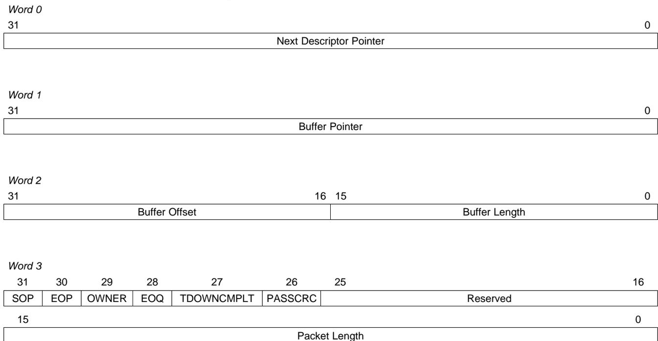
**Example 1. Transmit Buffer Descriptor in C Structure Format**
