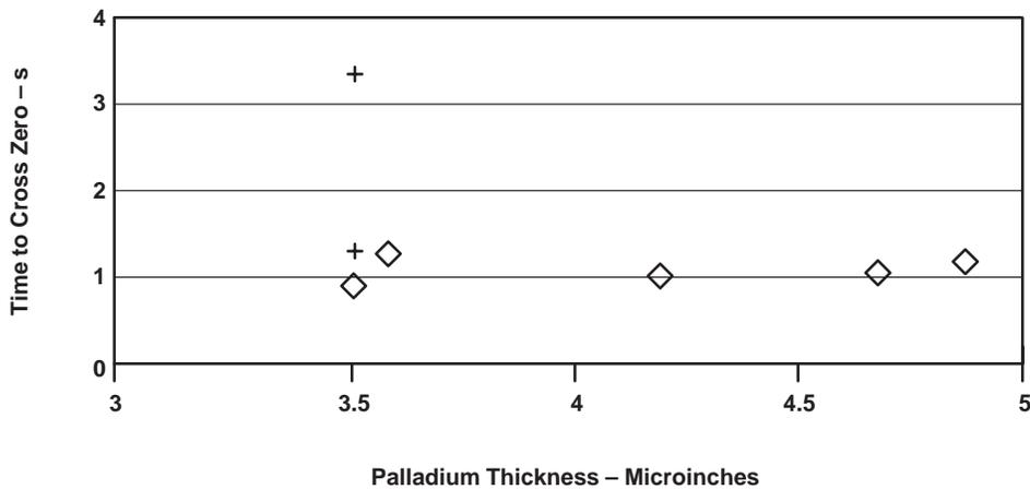
**Figure 8. Average Time to Zero vs Pd Thickness**
