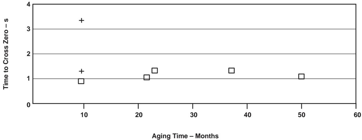
**Figure 7. Average Time to Zero vs Aging Time**
