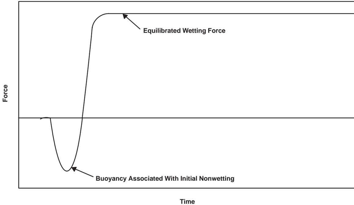
**Figure 6. Typical Wetting-Balance Curve**
