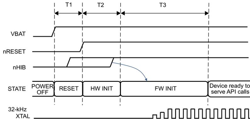
Figure 8-6. First-Time Power-Up and Reset Removal Timing Diagram
