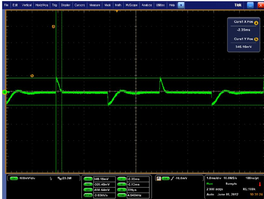
1A~11A step load, 1A/us slew rate, **x2 oversampling**
