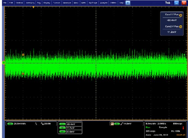
$V_{in}=48V$ ,  $I_o=10A$  /Ripple= $28mV$
