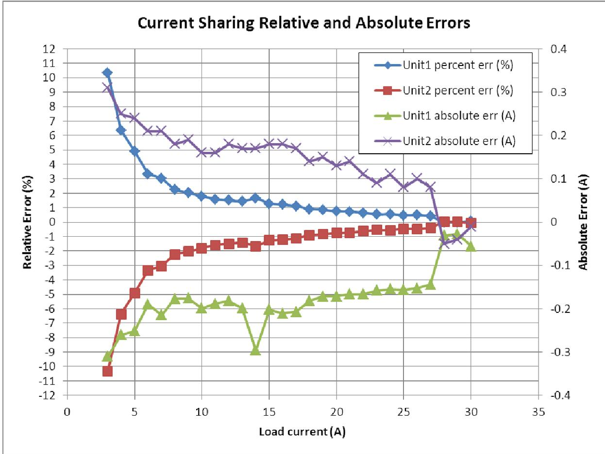
**Figure 4 Current Sharing Relative and Absolute Errors**
