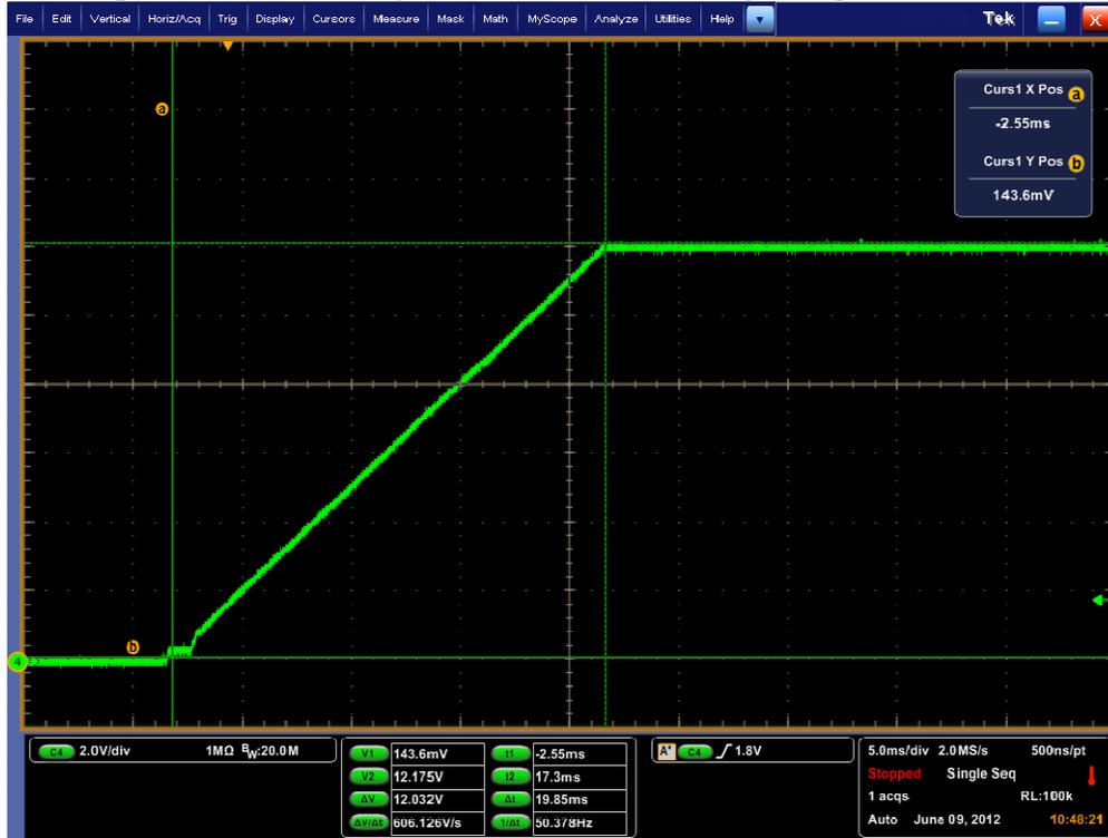
Soft start at 48V input, 10A load, with syncFETs on from the beginning
